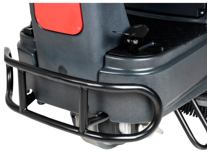
Front bumper protects the machine
